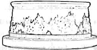
e) Recess on inner race
