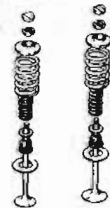
Fig. EM-34 Valve components
