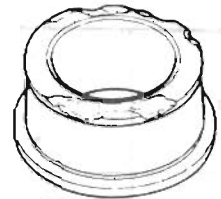
c) Cracked inner race
